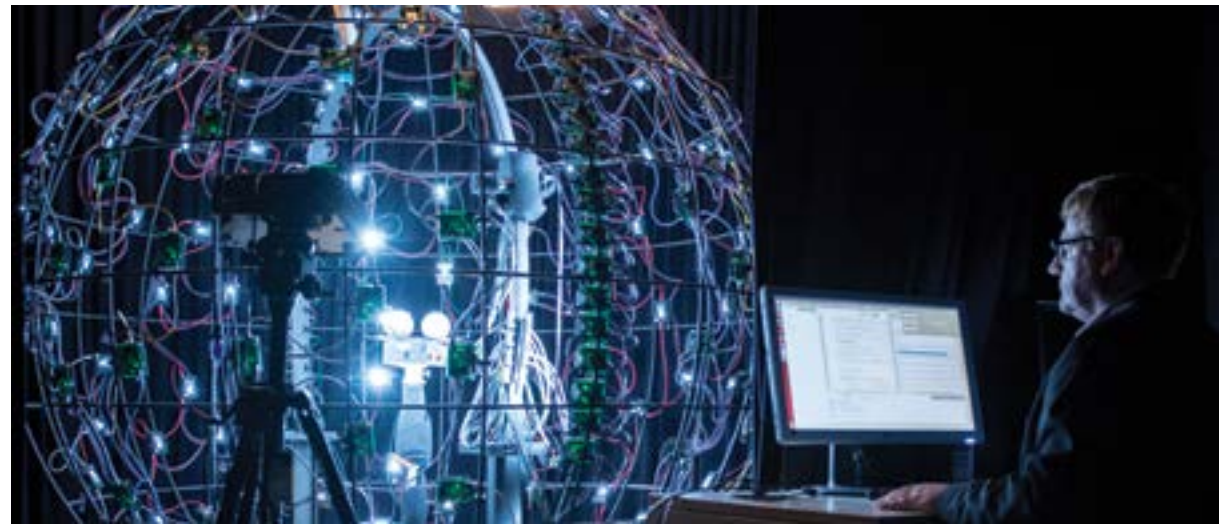
Professor Hendrik Lensch of the University of Tübingen is seated in front of a light stage, where he is conducting various computer graphics experiments. The hyperspectral light stage allows for precise acquisition of a reflectance field for a given scene by illuminating it from about 200 directions with a controlled spectrum, capturing HDR photographs and accurate 3D scans from almost any perspective.
