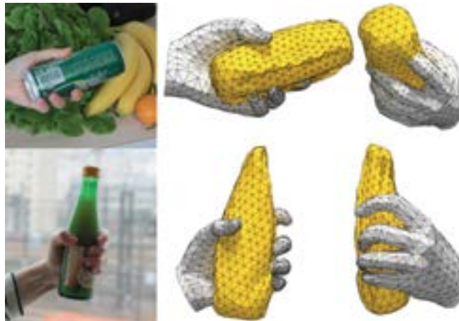
Reconstruction of realistic hand and object interactions by learning a model that estimates hand pose and shape together with object shape by enforcing physical constraints.
