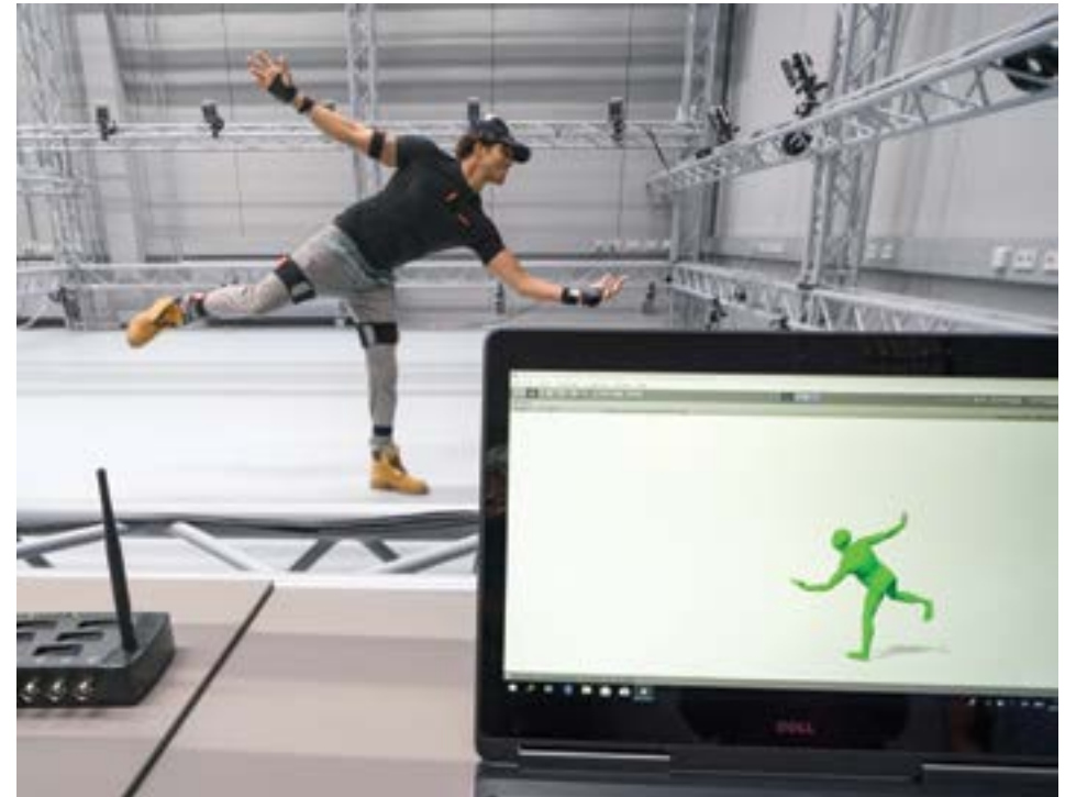
Sixty-six cameras record the person's movement, down to the last detail and millimeter. Of these, 22 record colour images, while the remaining 44 record black and white. Each camera captures 60 shots per second, for a total of 237,600 pictures per minute.
