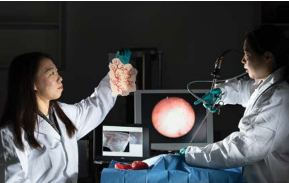
Human-like organ models are developed to test new medical instruments, provide quantitative evaluation on surgical performance and offer useful feedback for surgeons to improve surgical skills.
