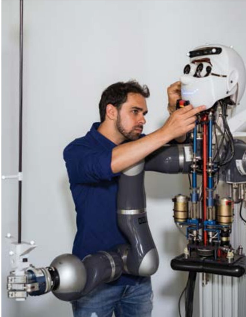
The robot Apollo tries to learn how to balance a rod. Using a camera system, the humanoid robot scans its surroundings 200 times per second, thus generating a 3D image of its surroundings and learning from what it sees. It then calculates how to move to balance the rod as perfectly as possible.
